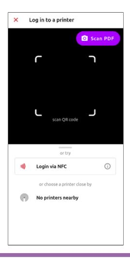
Only an administrator can pair an NFC tag to an MFD. Tap the Login button and then tap the information button 1 next to the Login via NFC option. Tap Pair new tag. Bring the phone close to the printer and tap Write to NFC tag. Once done, scan the QR code on the printer to finish the device pairing.
