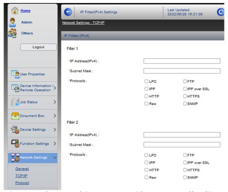
To ensure the proper function of the Device spool feature, turn off **IP filters** or **set a new IP filter** which includes all the IP addresses of the printing devices, where the pull print jobs can be stored.
